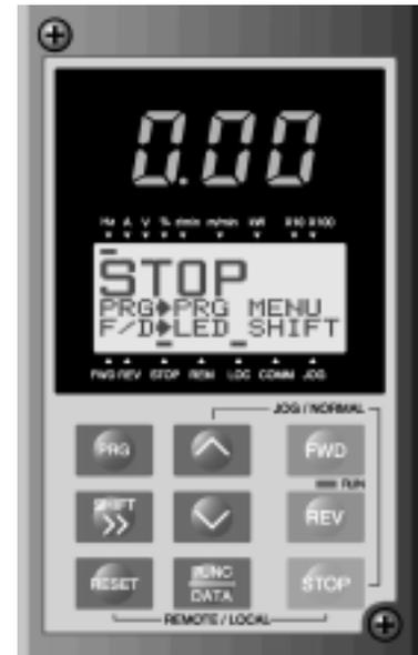
Fig. 3-1-2 Display on keypad panel at power-on
